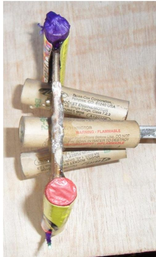
The first time I tried this, I used three high-thrust B-class motors as the spin motors. The ensuing RPM was slightly colossal: the pidgeon disintegrated due to centrifugal forces, and all three nozzles of the lift motors were also flung out due to centrifugal forces! So be warned, use only very low thrust spin motors, or cant them only a few degrees to create spin: a very slight turning moment is all that is required.
