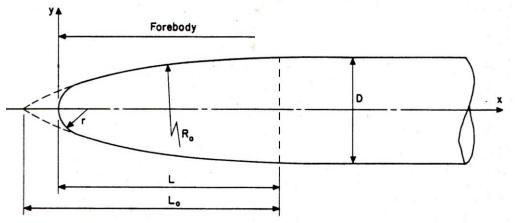
A nose cone formed by revolving a circular arc of radius  $R_0$  about the central *x* axis. The arc is tangent to the cylindrical fuselage at the nosecone base. Note that in this paper, the **fineness ratio** (length to diameter ratio) of the nosecone is based on *L* rather than the unblunted  $L_0$ . The majority of HPR nosecones are tangent ogives as they give adequate low drag performance and are easy to design.
