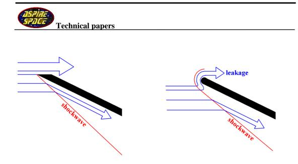
Sharp and blunt edge flow at angle of attack
