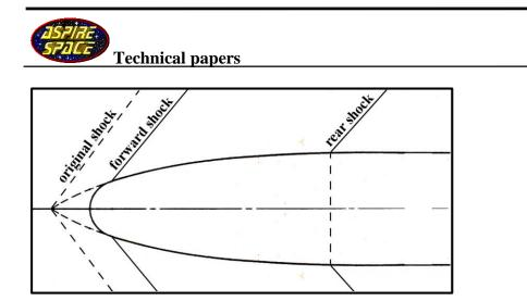
This forward shock as it were 'pulls the teeth' of the rearward shock, resulting in two shocks that are weaker than the original single shock. Weaker shocks give less wave drag.
