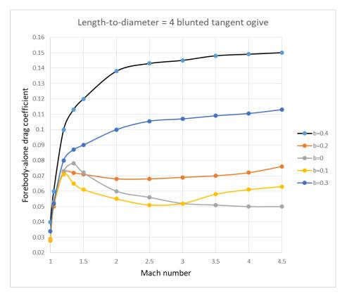
Note that these data are for the wave drag (pressure drag) of the **forebody** *alone*, assuming a perfectly aerodynamic afterbody and no viscous/boundary layer effects. Below about Mach 0.7 there are no shockwaves, therefore these curves drop to zero at Mach = 0.7
