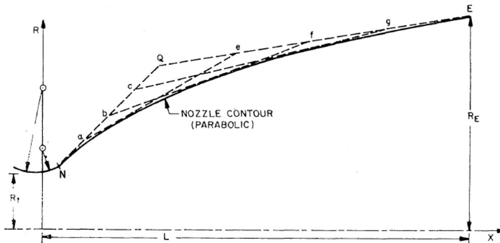
Straight lines are drawn at angles  $\theta_n$  from point  $N$ , and  $\theta_e$  back from point  $E$ , terminating where these lines cross at point  $Q$ .
