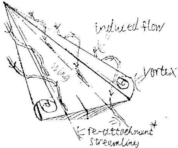
This spinning tame whirlwind induces flow above the vortex, which would otherwise be stalled at such a high angle of attack, to flow back down onto the wing. Also, the rapidly spinning vortex creates lift by speeding up this induced upper flow as it passes over the vortex, reducing its pressure.
