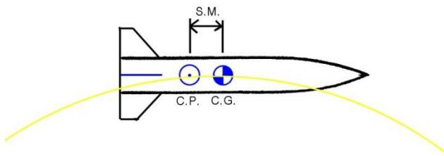
The tailfins are counteracting the lift of the nose, so that the overall centre of lift, which in rocketry we call the Centre of Pressure (C.P.), is behind the Centre of Gravity (C.G.) and so the rocket is aerodynamically stable (see our paper ‘Rocketry aerodynamics’ section 4, for details of stability). The distance between C.P. and C.G. is called the Static (stability) Margin (S.M.).
