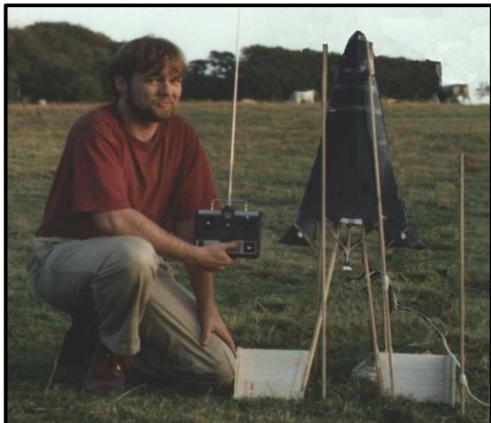
I've found that it's best to have a higher aspect ratio on the fins than the glider, so that the fins have a steeper **lift curve slope** for added static stability.
