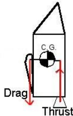
Because the thrust is such a large force, even a small moment arm (a near-miss) can cause a looping flight.
