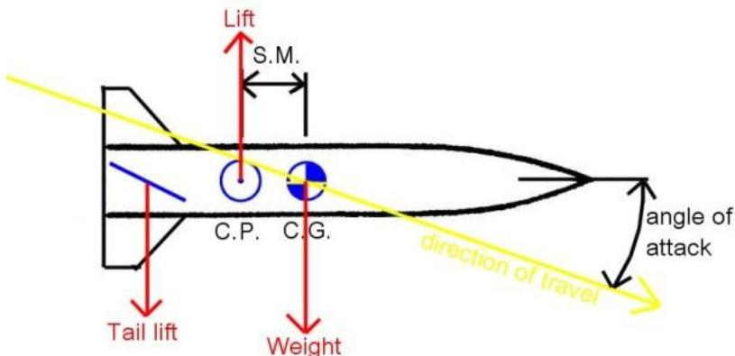
Now the vehicle is gliding: the direction of travel (of the C.G.) is shown here in yellow. The C.P. and C.G. are not coincident (finite Static Margin for stability) but this unfortunately creates a nose-down pitching moment (called a ‘couple’) in the pitch axis: the lift and the weight are pulling in opposite directions, but are some distance apart.
