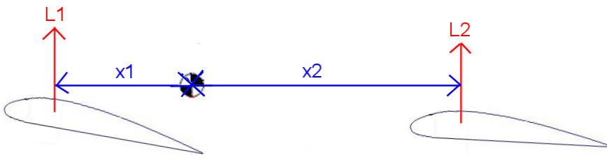
The forward wing is bolted-on at double the angle of attack of the rear, so is lifting with double the force of the rear. Therefore the C.G. (pivot of the see-saw) has to be nearer the front wing to keep balance: distance  $x_1$  is half of distance  $x_2$ .
