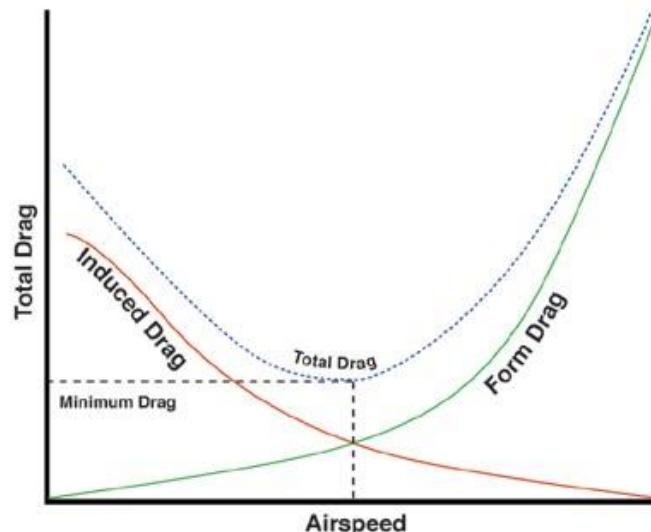
With traditional aircraft (no leading-edge sweepback) the minimum drag airspeed is just above the level-flight stall airspeed, so pilots rarely find themselves flying below this airspeed. This is just as well, because flying below the minimum drag airspeed, which is called 'flying on the back-side of the drag curve' can be very confusing.
