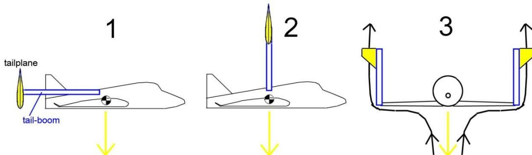
But this would mean that the tailplane would be in the dead air of the wake; it wouldn't work. At this point I gave up, but Burt didn't. He realised that he could modify the tailboom of picture 2 by splitting it in two and bolting it to the wingtips. As the front view of picture 3 shows, the tailfins are now in the moving air flowing past the vehicle so will function properly. And that's why Burt is a genius!
