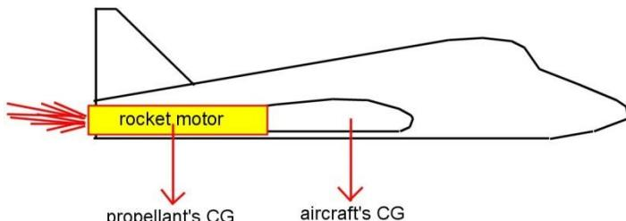
However, as propellant is jettisoned out the nozzle, the remaining propellant mass decreases, and unfortunately, the propellant's own C.G. is significantly rearwards of the overall aircraft C.G. So the tail gets progressively lighter, making the aircraft progressively nose-heavy (the overall C.G. moves nosewards), which requires more and more elevator deflection to keep in trim and prevent a nosedive. The required elevators can get excessively large and draggy.
